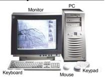
Used for processing, storing, displaying, etc. of image data obtained by X-ray CT, MRI, PET-CT, etc.
